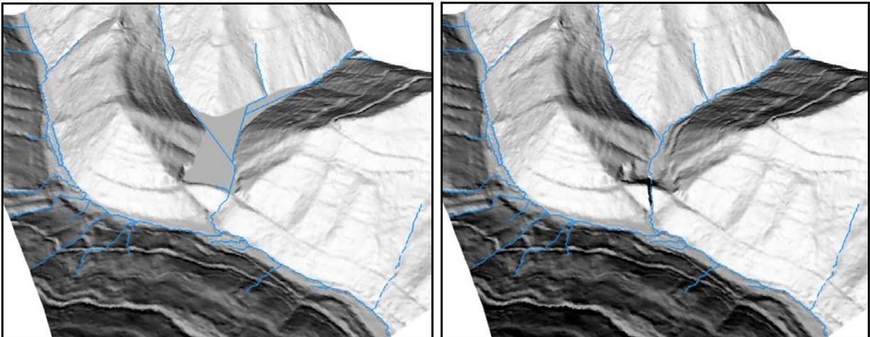
Figure 9. An abandoned railway line produced a false 'lake' during processing to extract drainage features (right). The fill had to be breached in order to accurately depict drainage above the apparent obstruction (left).
