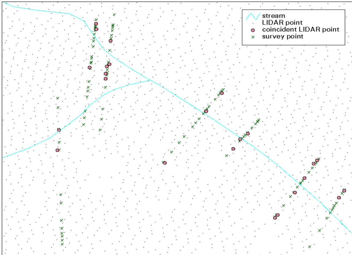
Figure 4. Coincident LIDAR points selected for evaluation based on proximity to survey points, section of Scrabble Creek.
