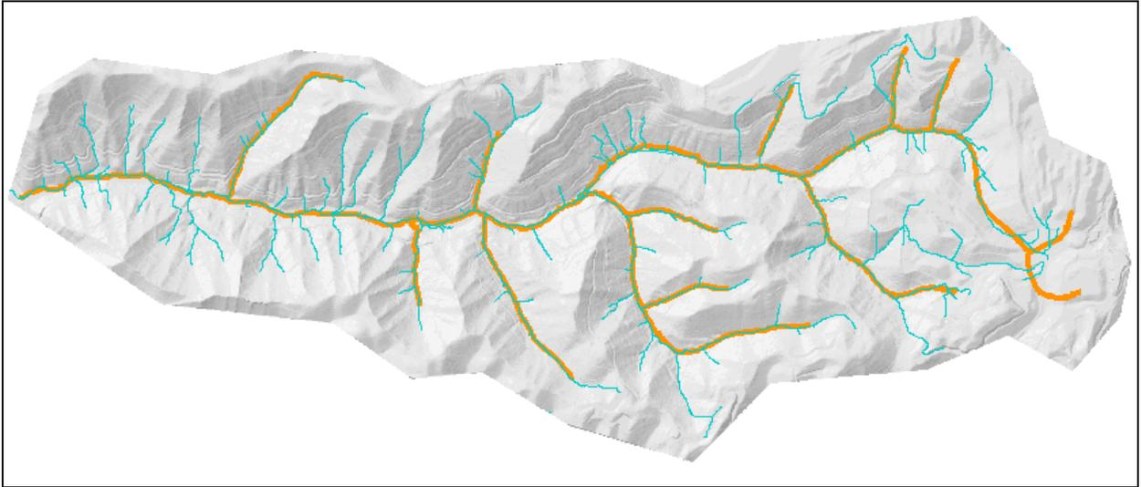
Figure 8. 4-acre drainage channels extracted from the LIDAR-derived grid, compared with 1:24,000 streams in yellow.
