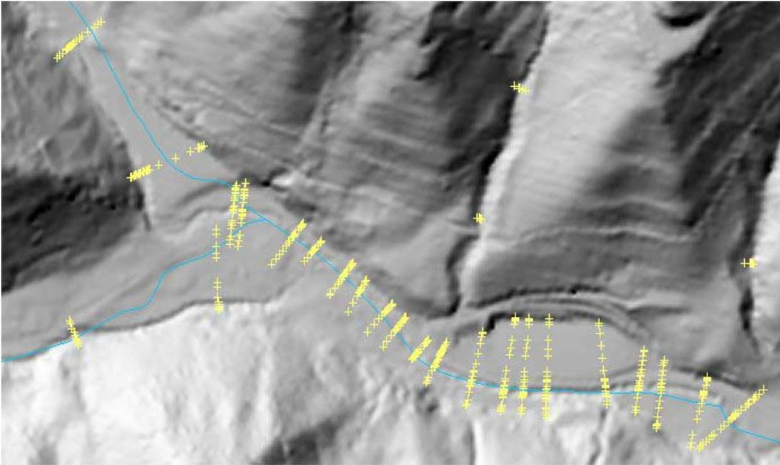
Figure 3. Field survey transects for a portion of Scrabble Creek Watershed, with LIDAR-derived hillshade as backdrop.
