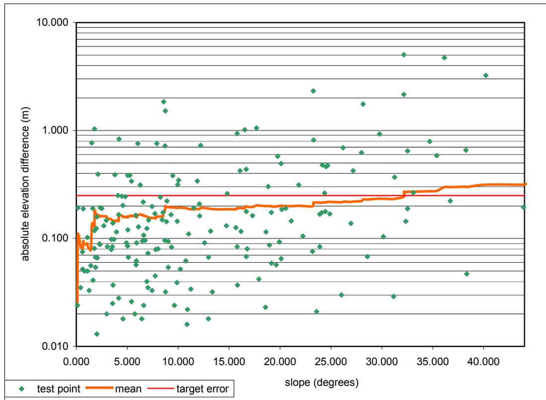
Figure 6. Relationship between slope and absolute elevation difference for coincident points in Scrabble Creek watershed.
