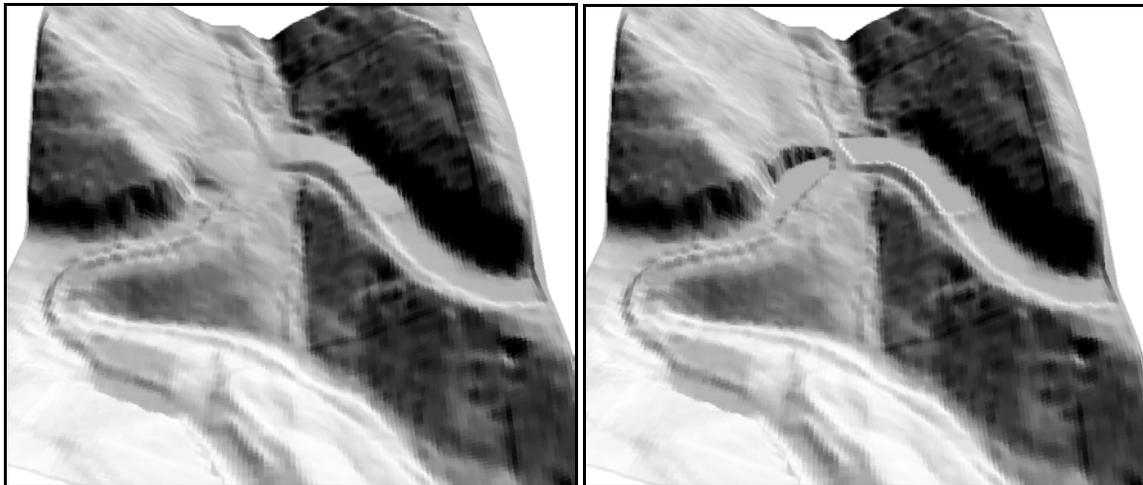
Figure 7. Errors produced by gaps in LIDAR data for waterbodies (left) can be corrected using breakline polygons (right) during the TIN creation process.
